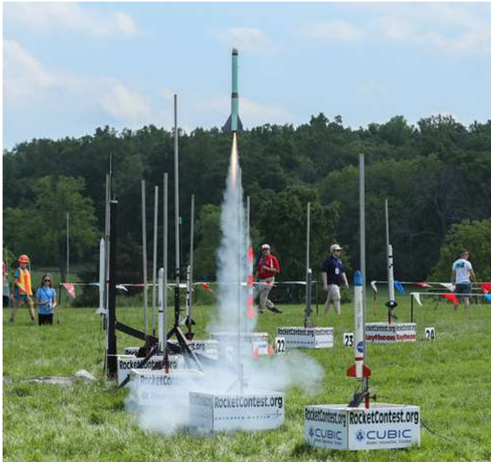
Figure 1-1. Rail launchers are frequently used to provide launch guidance for large model rockets.
