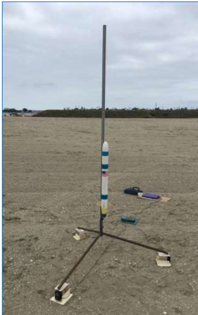
Figure 6.1-1. Vertical force in the rail launcher was measured using three force sensors (one under each leg).
