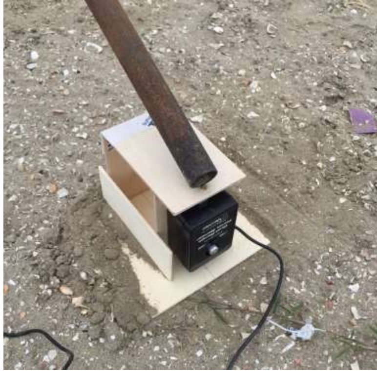
Figure 6.1-2. A force sensor was placed under each leg of the rail launcher.
